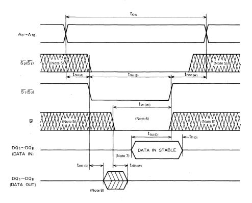
Note 4: Test conditions Input pulse level: 0.4 ~ 2.4V Input pulse risetime and falltime: 10ns Load: 1TTL, C<sub>L</sub> = 100pF Reference level: 1.5V
